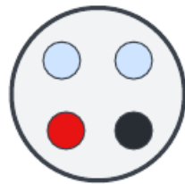
4x 18 AWG Conductors, 2 for Power, 2 for 10BASE-T1L Data
