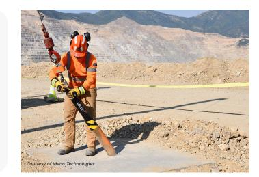
Ideon Technologies is a pioneer in cosmic-ray muon tomography, enabling x-ray-like imaging up to 1 km underground. In an accelerated development schedule of 12 months, MistyWest developed the next generation of Ideon's muon detector, miniaturizing a benchtop system from 1x1x1m to a rugged, manufacturable Ø10cm by 3m form factor. 10 field-deployable prototype muon detectors were delivered that can operate reliably for months without failure.
