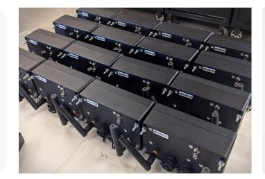
Guide Robotics develops SLAM-based navigation and robot autonomy technology for optimizing industrial operations. MistyWest was asked to redesign a rugged, compact, thermally managed device for mounting to forklift overhead racks, while eliminating the 10% failure rate of their existing device's power converter.
