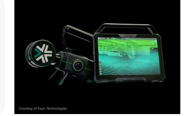
Exyn Technologies is commercializing LiDAR-based 3D mapping and autonomous navigation. They approached MistyWest for conceptual designs of a new commercial device that combined their existing handheld product ExynPak with their drone-mounted ExynAero product line.
