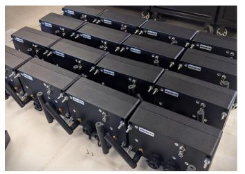
Guide Robotics develops SLAM-based navigation and robot autonomy technology for optimizing industrial operations. MistyWest was asked to redesign a rugged, compact, thermally managed device for mounting to forklift overhead racks, while eliminating the 10% failure rate of their existing device's power converter.
