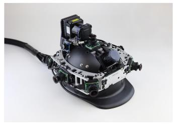
A startup bringing VR technology to commercial real estate engaged MistyWest to develop a novel 3D mapping camera designed to capture high-resolution spatial data, requiring integration of seven high-resolution cameras into both an existing helmet design and a custom triggering system.
