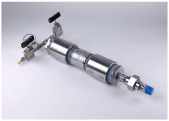
After taking over the experimental operation of the system, Rockburst Technologies and <u>UBC Mining</u> were able to successfully and safely demonstrate ~50% energy reduction. The industrial apparatus continues to demonstrate the technology of pulverizing rock with transcritical CO<sub>2</sub>, aiding Rockburst in securing investment for future development.
