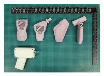
Cannabix Technologies Inc. partnered with MistyWest to develop a THC breathalyzer prototype for law enforcement. MistyWest engineered a Breath Collection Unit (BCU), optimizing airflow geometries, designing foam models for UX testing, and developing a companion Android app for real-time data via Bluetooth. Within a short timeline, we delivered two fully functional prototypes capable of measuring breath volume, CO2 content, temperature, and humidity.
